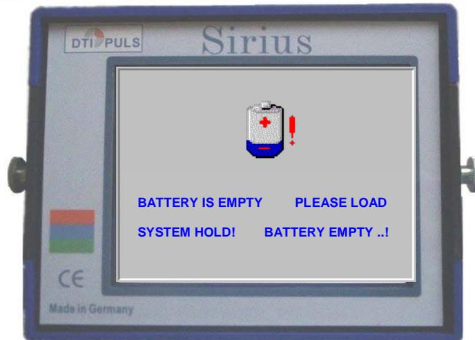
The condition of the rechargeable batteries will be checked. If the rechargeable battery is not ready for operation a message will be displayed. You have to switch off the detector for charging batteries.
