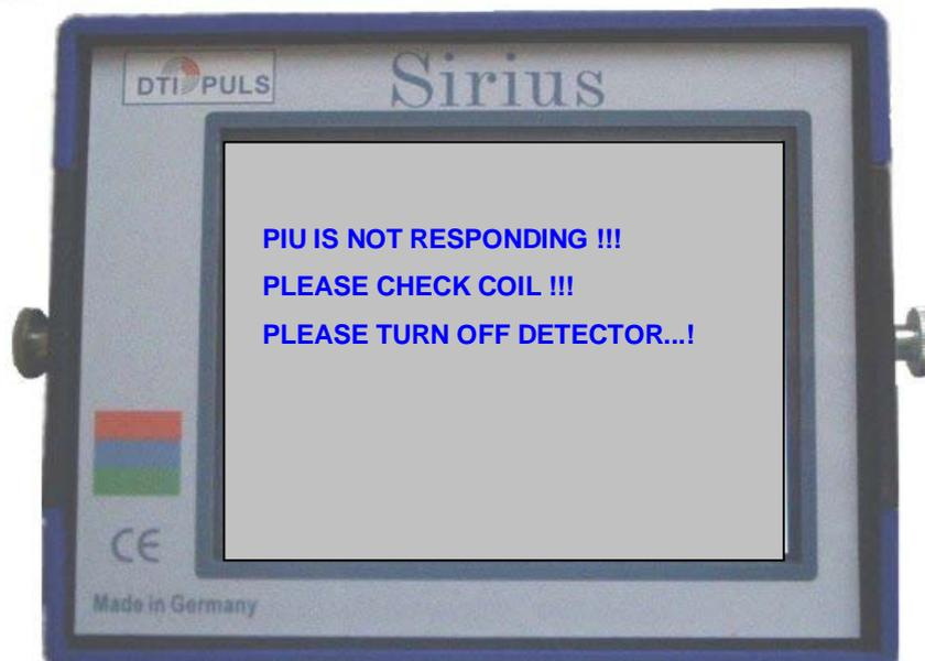
In case of a problem with the communication of both internal processors it can happen that the wrong data is being used. That can happen because of some influence from outside of by switching on and off in a short time by accident. In this case please switch off.
