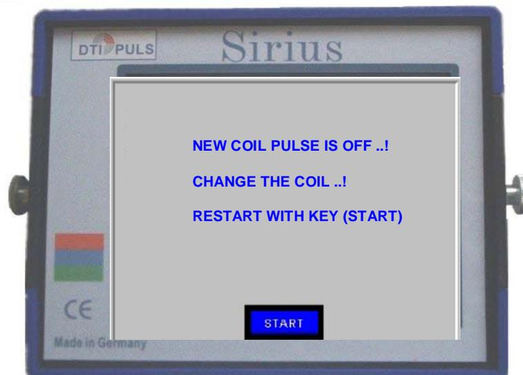
You will now be able to change the coil when the detector is switched on. Only if you see this message, changing is allowed. Afterwards the instrument only needs some time for stabilizing the coil. If you change from a higher power coil to a lower power coil the power will be adapted, but not rise again automatically if you go back to a higher power coil. So you should store the settings before changing.
